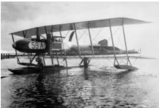
Experimental Gallaudet, propeller in the fuselage 1061646
