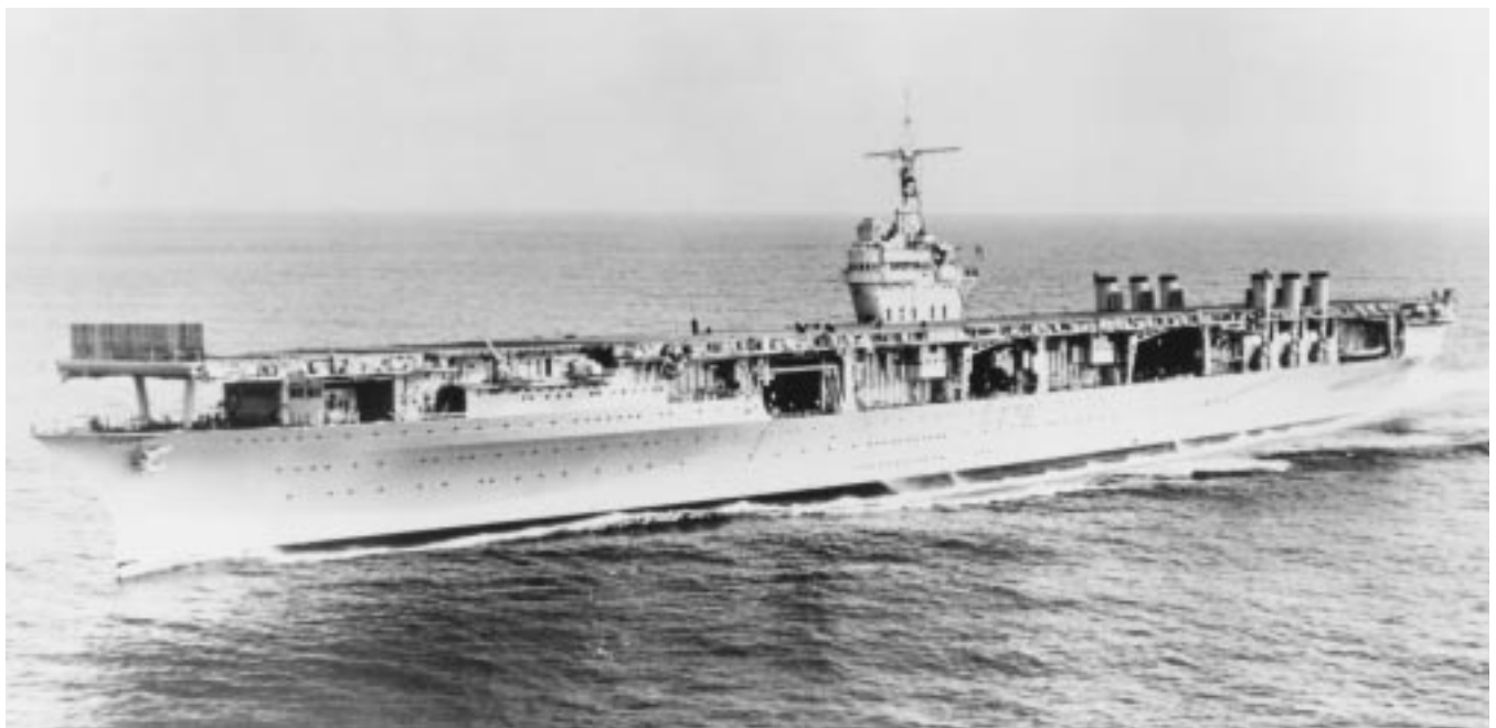
The 14,500-ton Ranger, CV-4, was the first American ship designated as an aircraft carrier from the keel up 428440
