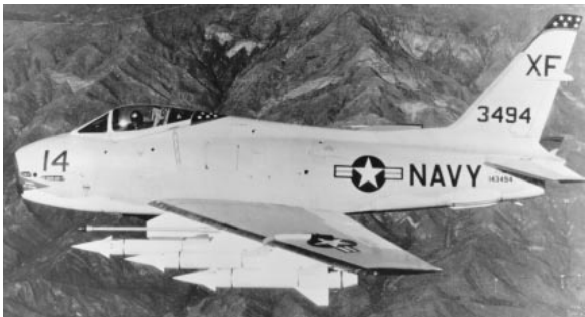
Bullpup air-to-surface missiles are carried by FJ-4B 710127
