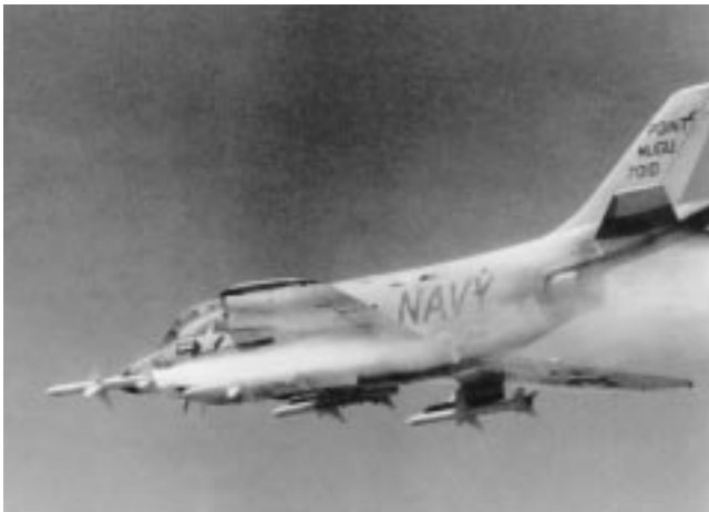
An F3H-2N firing air-to-air Sparrow III missiles 1061490
