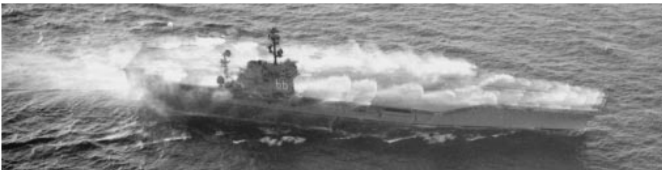
Light water in washdown system, used for fighting fire
