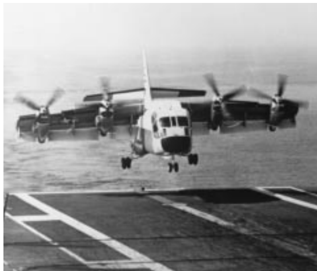
The XC-142A vertical takeoff and landing aircraft during trials aboard Bennington NH 69968
