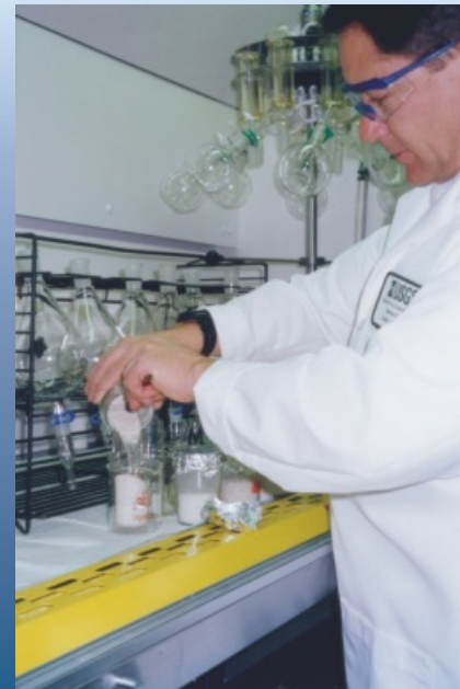
Fish-tissue samples are prepared for Soxhlet extraction.
