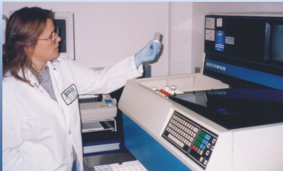
Sample vials of ambient water in a scintillation cocktail are loaded into a liquid scintillation system for radon detection.
