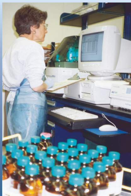
Dissolved organic carbon samples are analyzed on an ultraviolet persulfate total organic carbon analyzer.
