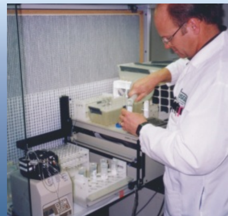
Samples of inorganic trace elements are prepared for analysis by inductively coupled plasma-mass spectrometry.
