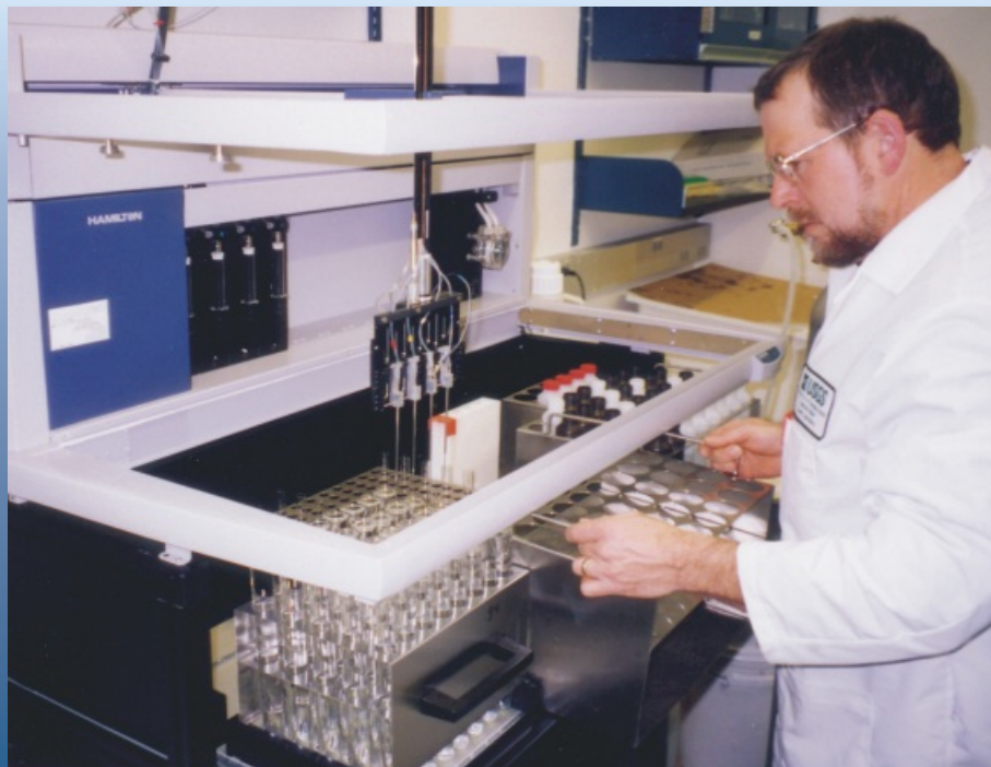
Robotic liquid sample-handling system is configured for automatic, simultaneous preparation of digests for dissolved Kjeldahl nitrogen and dissolved low-level phosphorus determinations.
