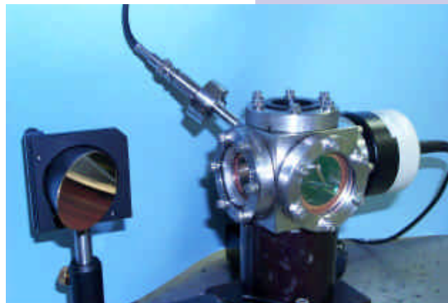
LLNL VOC test chamber with achromatic free space focusing. [see Project #70050]
