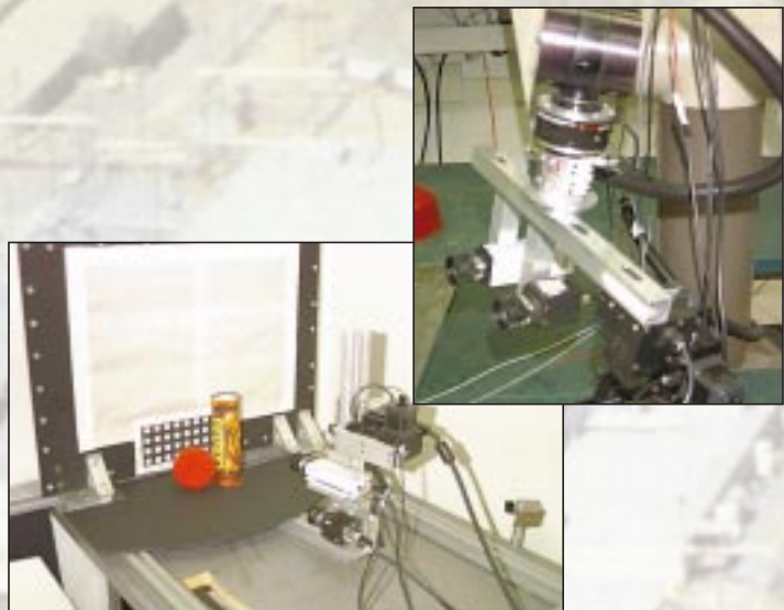
▲ Laser and camera setup during one of the initial system tests demonstrating the compact size of the scanners.
