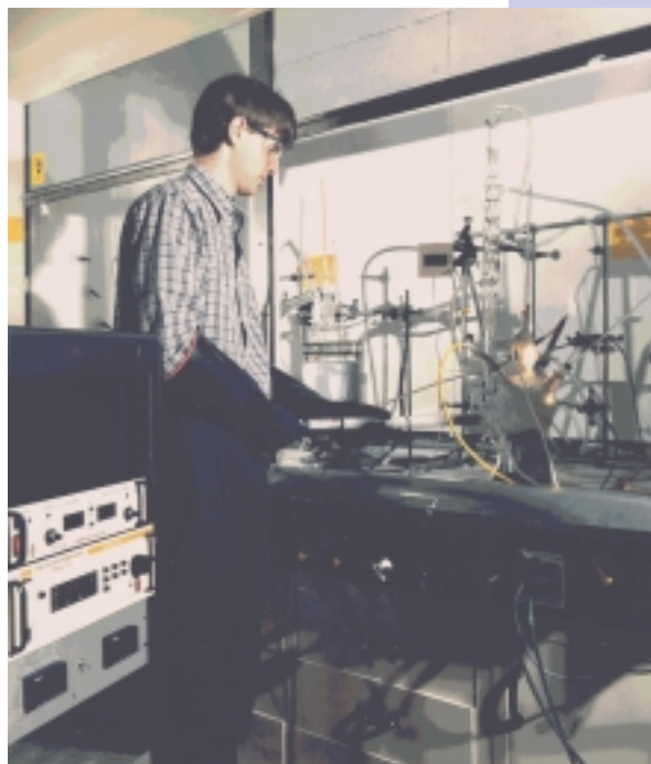
Phase equilibria and interfacial transport may be modified to enhance separations by applying an electric field. A vapor-liquid-equilibrium experiment is shown here. [see Project #55119]
