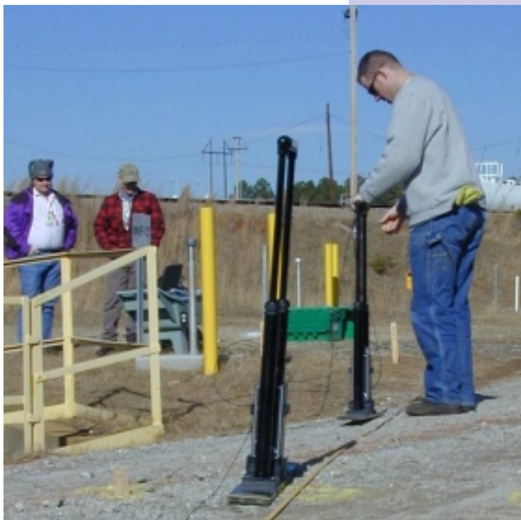
Multi-offset, ground-penetrating radar data acquisition for DNAPL detection at the SRS. [see Project #70052]
