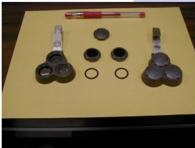
The insides of the radon-222, radon-220 monitor device. [see Project #74050, renewal of #59882]
