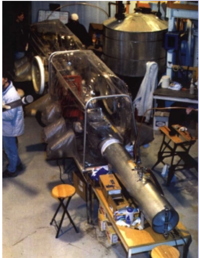
Aseptic sampling of fractured rock. [see Project #55416]
