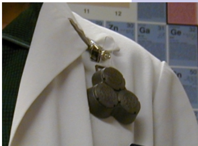
Radon thoron detector, as it would be used in the field of personal monitoring. [see Project #74050, renewal of #59882]
