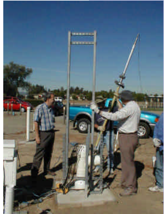
Researchers with the new Electromagnetic Induction Tomography (EMIT) tool, designed for subsurface characterization of a contaminated site. [see Project #70149, renewal of #54950]
