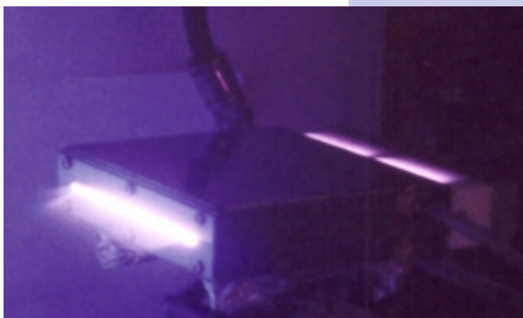
Front view of a 4" wide thermospheric-pressure plasma source operating with 750 Torr helium and 10 Torr oxygen. [see Project #73835, renewal of #54914]
