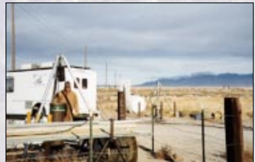
Seismic recording van and receiver well with tripod
