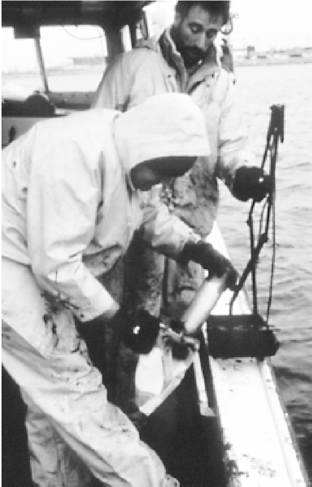
Sampling contaminated dredge material in Boston Harbor, MA.
