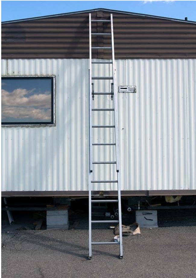
Exhibit 2-1, Ladder base at 3 ½ feet from MO-392, south wall.
