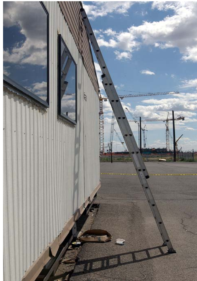
Exhibit 2-2, Ladder base at 3 ½ feet from MO-392, south wall
