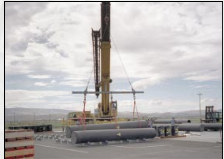
Mixed low-level waste debris is "macroencapsulated" in high-density polyethylene tubes.
