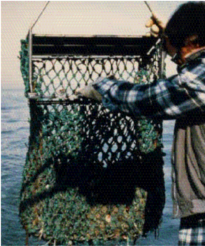
Shellfish and sediment samples are collected in estuarine and coastal areas to test for the presence of many different types of toxic chemicals.
