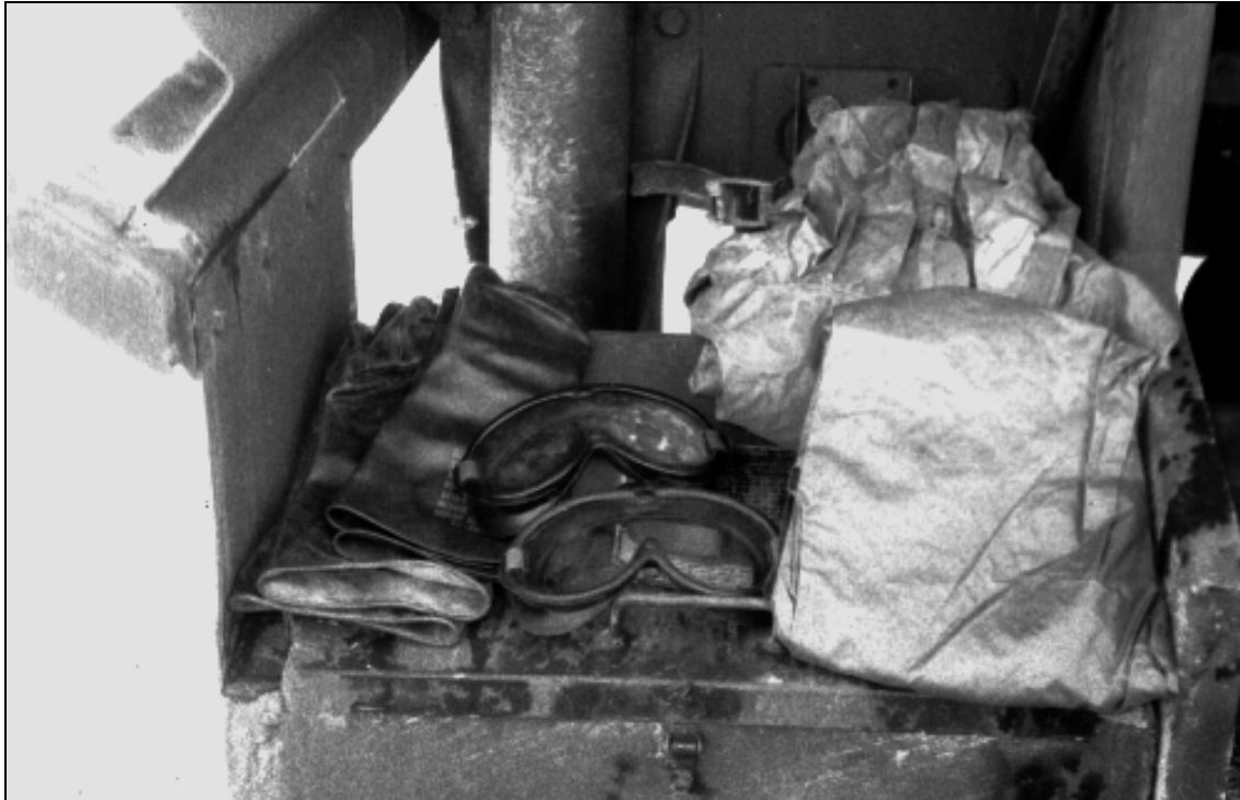
Figure 7: Personal protective equipment is the primary means of safeguarding human health when conducting tactical refueling operations. Goggles and butyl rubber gloves must be worn when conducting filling operations, and aprons or wet weather gear must be readily available to respond to a spill or repair a leak. More appropriate PPE can be obtained by referencing MSDSs.
