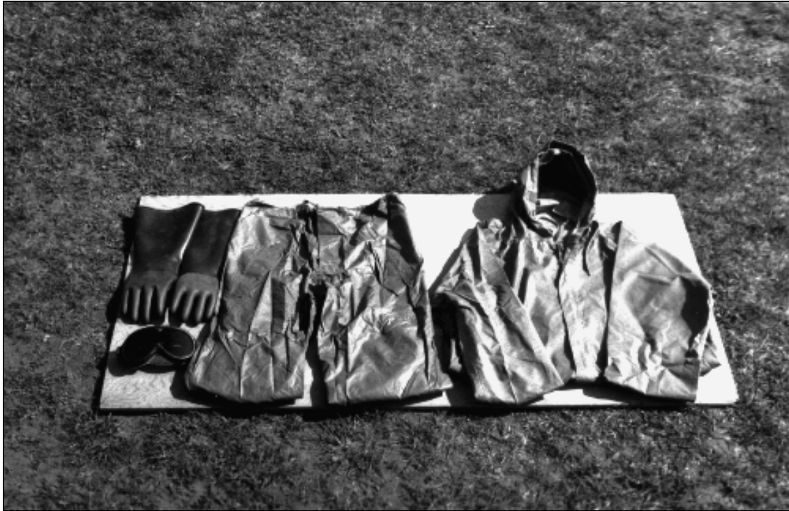
Figure 3: Personal protective equipment is the primary means of safeguarding human health when handling HM/HW. Appropriate field expedient PPE for HM/HW storage sites consists of field or butyl rubber gloves, goggles, and wet weather gear, as illustrated above. More appropriate PPE can be obtained by referencing MSDSs.
