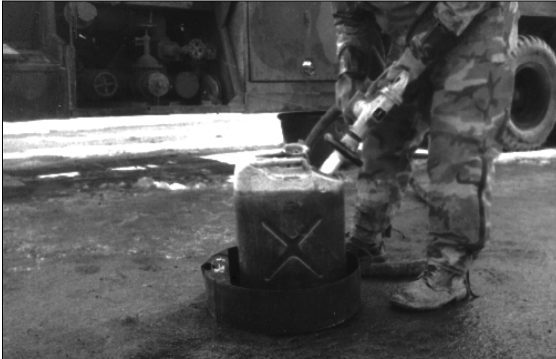
Figure 6: POL section personnel need to ensure that 5-gallon fuel cans are placed inside of an appropriate secondary containment device as illustrated above. When filling the fuel cans, 1.5-2 inches of headspace is required to allow for vapor expansion. All spilled fuel must be immediately transferred to a "Waste Fuel" collection container for proper disposal.
