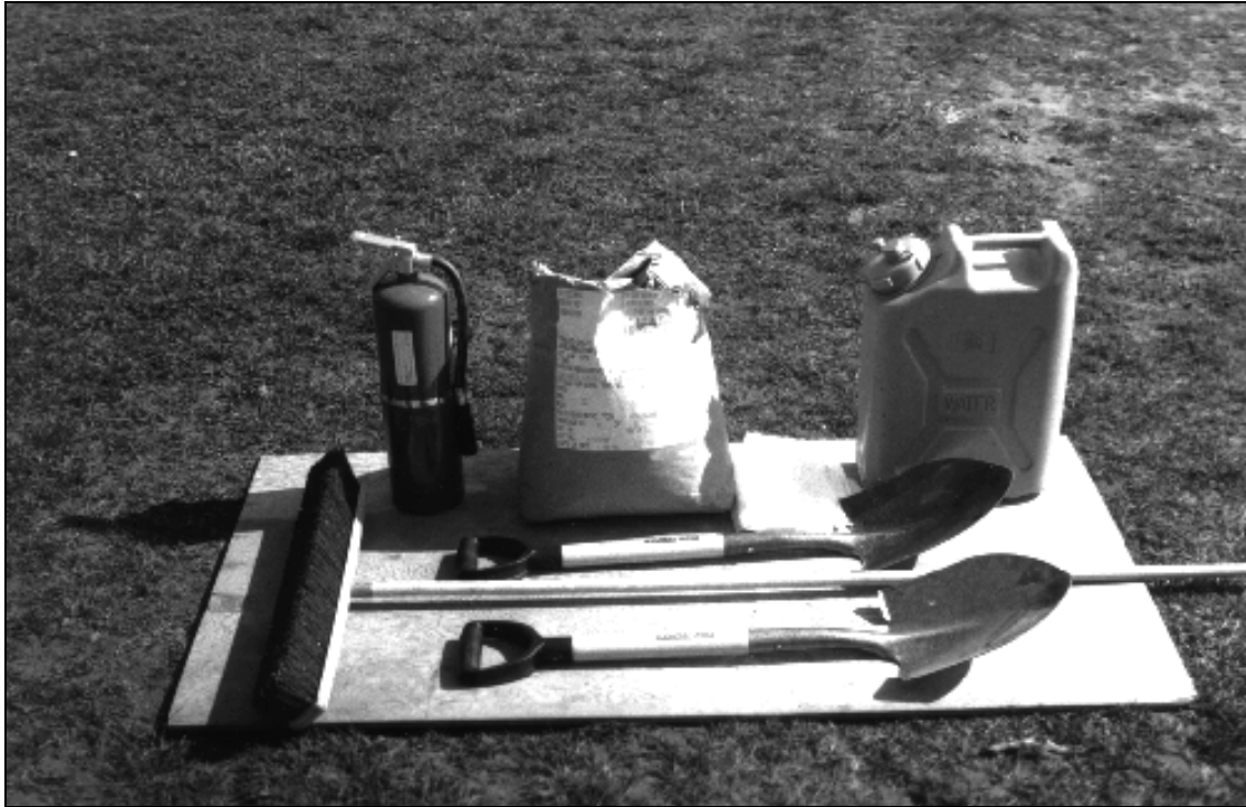
Figure 4: Emergency equipment is essential for properly responding to HM/HW incidents. As illustrated above, the appropriate equipment for HM/HW storage operations consists of an ABC fire extinguisher, potable water for emergency eye-washing, and absorbent, shovels, brooms, and plastic bags for spill response.
