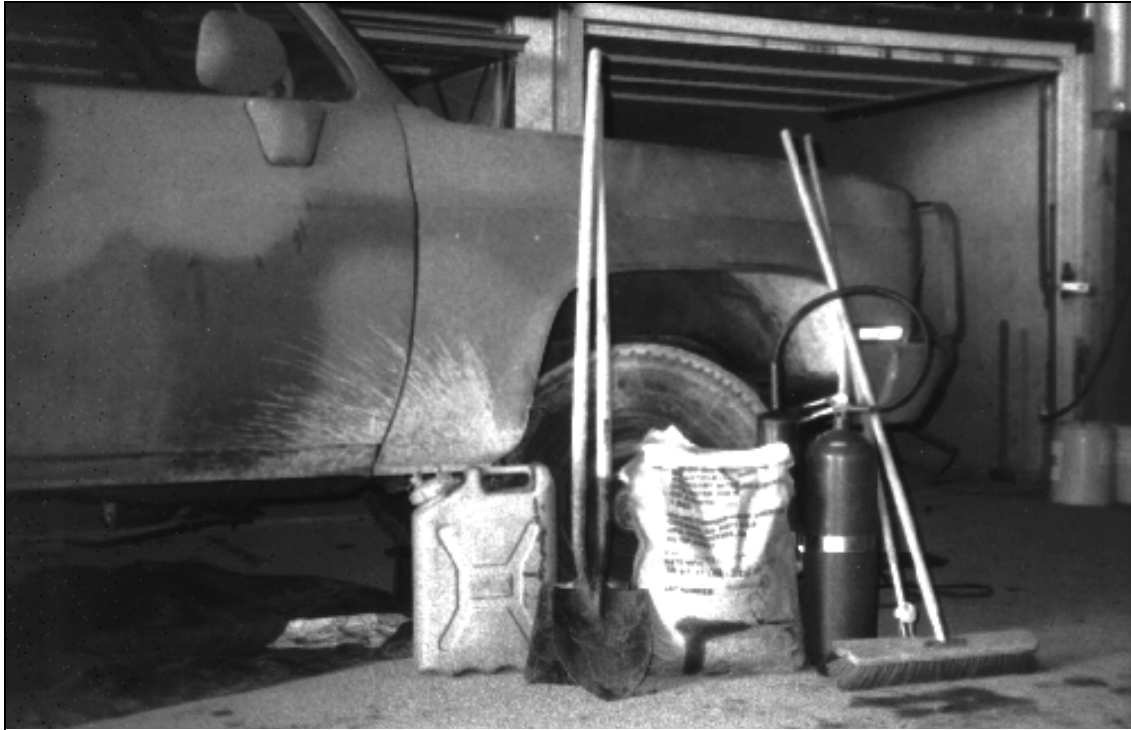
Figure 11: Emergency equipment is essential for properly responding to HM/HW incidents while conducting field maintenance operations. As illustrated above, the appropriate equipment consists of a fire extinguisher, potable water for emergency eye-washing, and absorbent, shovels, brooms, and plastic bags for spill response.
