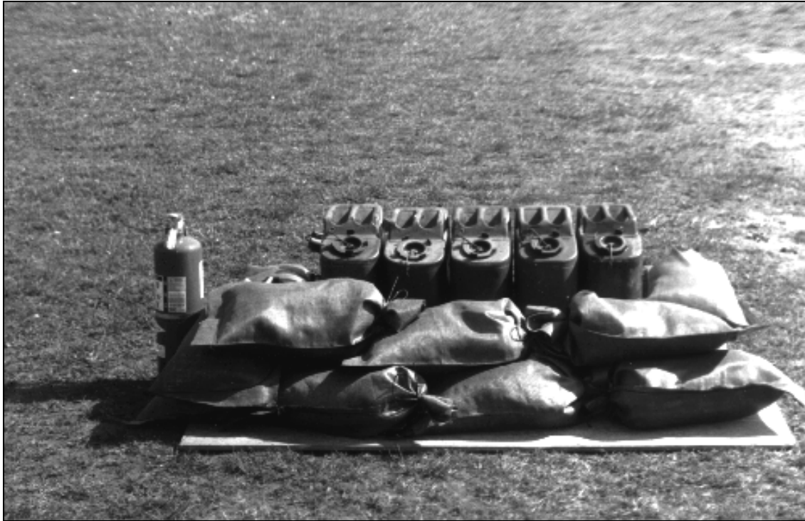
Figure 2: Fuel cans need to be consolidated and properly stored within each company or platoon AO. Proper storage consists of a piece of plywood and a sand bag perimeter large enough to hold 10% of the overall volume stored, as illustrated above. A tarp or plastic liner can also be used in place of the plywood.
