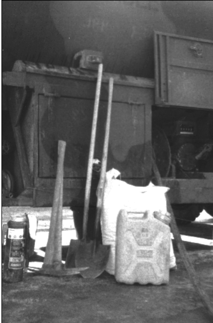
Figure 8: Emergency equipment is essential in responding to refueling incidents. As illustrated above, the appropriate equipment for tactical refueling operations consists of fire extinguishers, potable water for emergency eye-washing, and absorbent, pick, shovels, and plastic bags for spill response.
