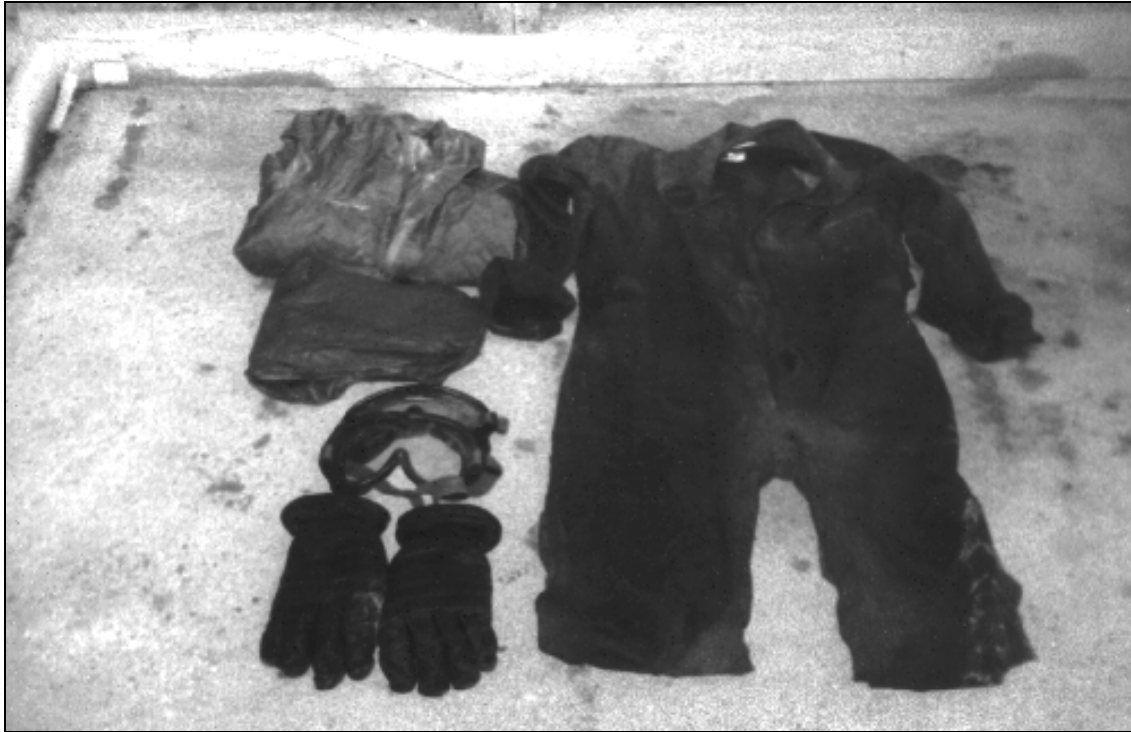
Figure 10: Personal protective equipment is the primary means of safeguarding human health when conducting maintenance operations. As illustrated above, the appropriate field expedient PPE consists of field gloves, goggles, coveralls, and wet weather gear. More appropriate PPE can be obtained by referencing MSDSs.
