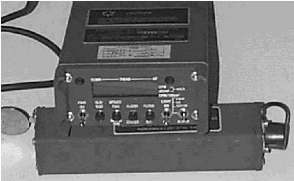
Figure 6: Picture of the AN/PDR-77 with the beta/gamma probe, Model DT 616.
