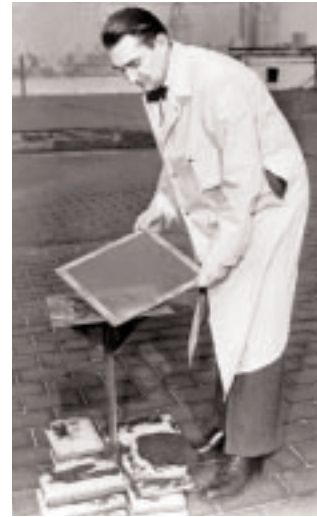
Gummed filter sampler on rooftop of USAEC Health and Safety Laboratory (now DHS/EML)
