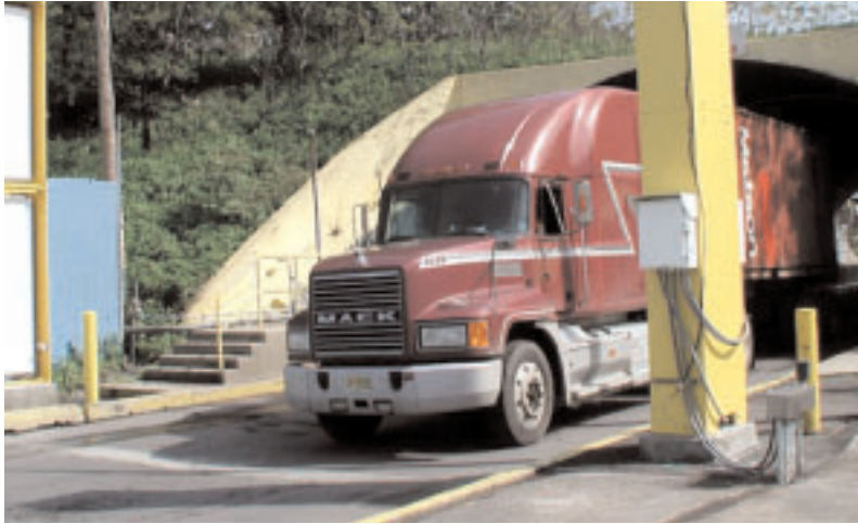
Test-bed venue deployment of radiation portal monitors
