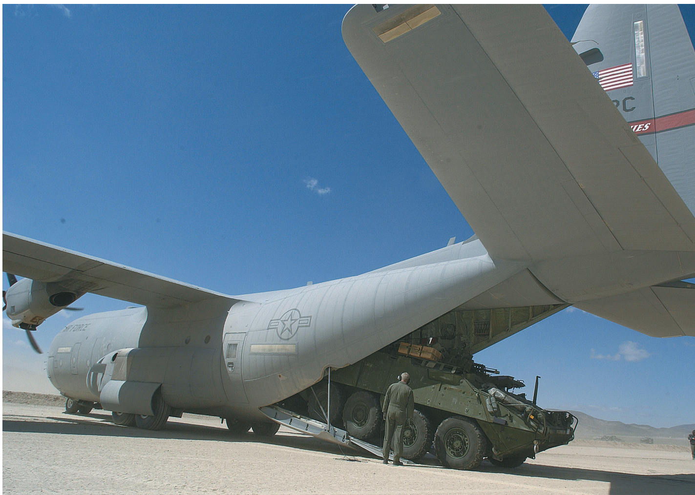
A Stryker mortar carrier exits the tail of an Air Force C-130 Hercules aircraft after landing at the National Training Center, Fort Irwin, Calif. (Army photo)
