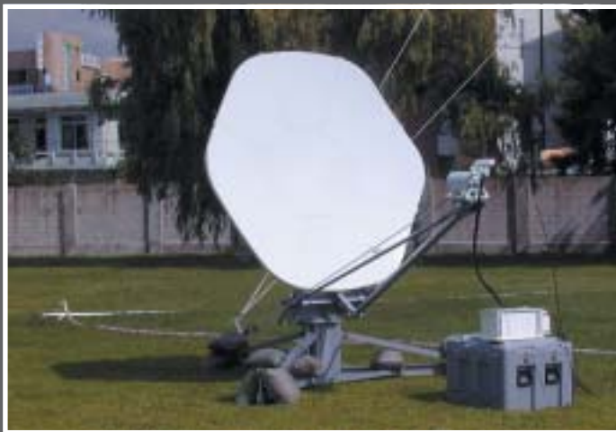
□ The collapsible 2.4-meter satellite dish used with the Multimedia Communications System.
