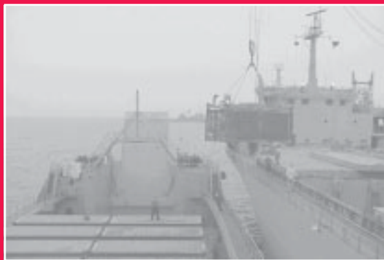
□ A container is transferred from the SS Cornhusker State to the smaller LTG William B. Bunker .
