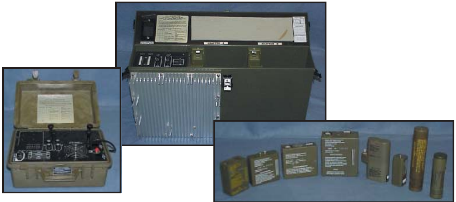
□ To facilitate the use of rechargeable batteries in tactical applications, CECOM developed a universal battery charger (left), a charger-on-the-move (center), and a new family of rechargeable batteries (right).
