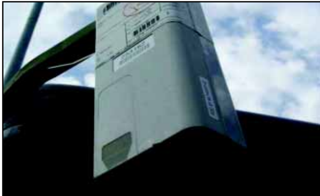
❑ Radio frequency transmitters are attached to cargo containers to help logisticians account for containers anywhere in the world.
