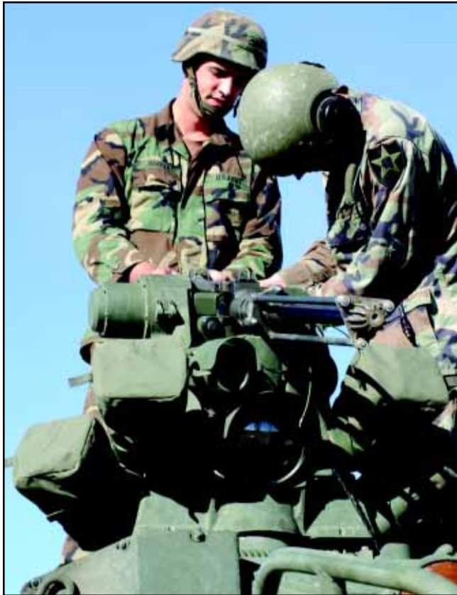
□ A soldier checks the Multiple Integrated Laser Engagement System strips on his Stryker armored vehicle before participating in Millennium Challenge 2002.
