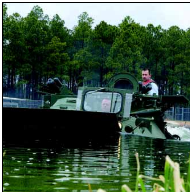
□ At Marine Corps Logistics Base Albany, Georgia, technicians test a light armored vehicle in the test pond located near the maintenance center.
