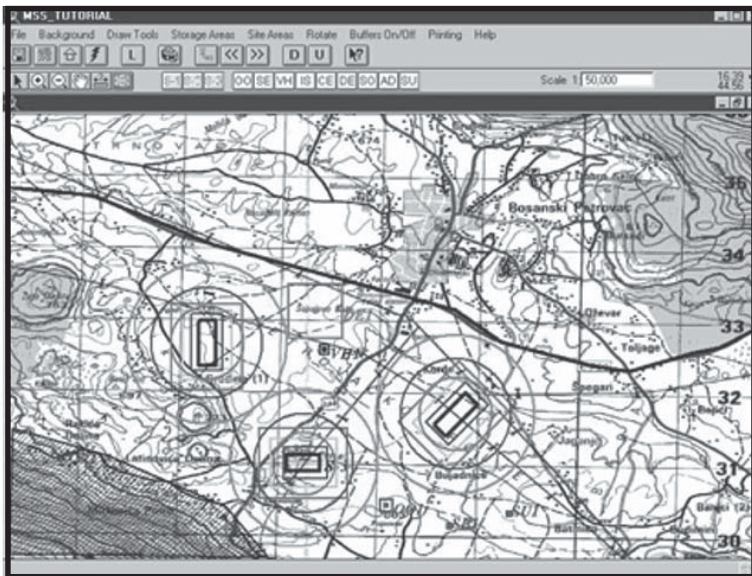
□ An ASA template developed using MSS can be placed over a military map to show the exact locations of the storage areas.
