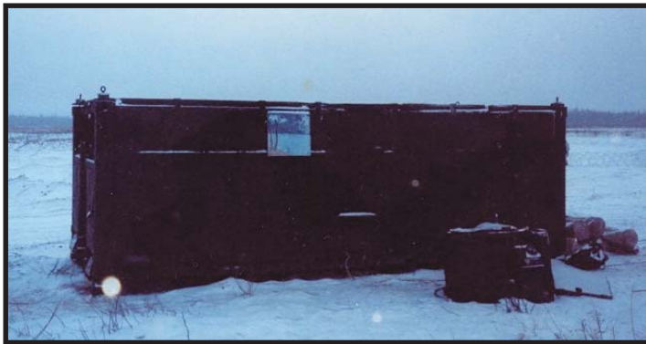
□ The "Arctic Oasis" is actually a covered flatrack that holds two 500-gallon water blivets and associated pumps and hoses.
