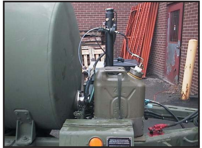
□ An innovative system to heat the contents of "water buffaloes" uses about 5 gallons of fuel in 48 hours.
