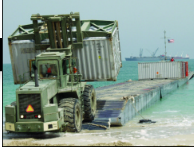
A rough terrain cargo handler unloads ammunition at Kuwait Navy Base during logistics-over-the-shore operations. Photo by Photographer's Mate Third Class Aaron Pineda, U.S. Navy, provided to Army Logistician by Captain Bobby Hart, 143d Transportation Command, U.S. Army.
