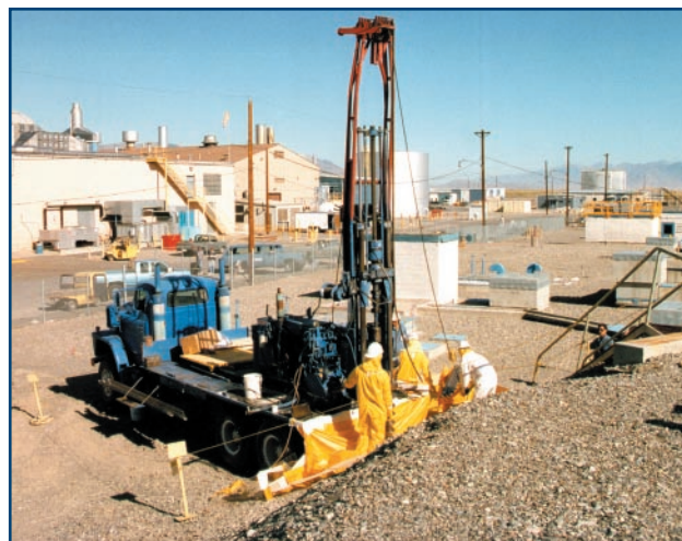
Figure 21. Soil is sampled at the INTEC tank farm to determine the nature, extent, and spread of contamination.
