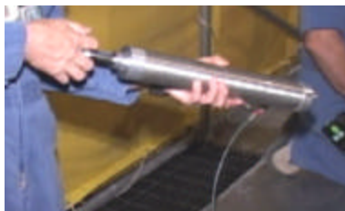
The Tank Heel Sampler was deployed in tank WM-182 to retrieve liquid samples for tank closure
