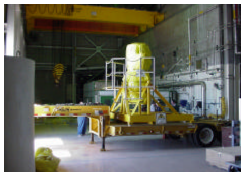
Spent nuclear fuel from the Material Test Reactor canal is prepared for shipment to dry storage at the Idaho Nuclear Technology and Engineering Center.
