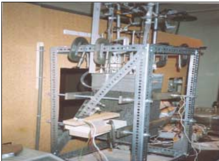
Figure A-5. Laboratory apparatus for measuring hydrologic properties of basalt.
