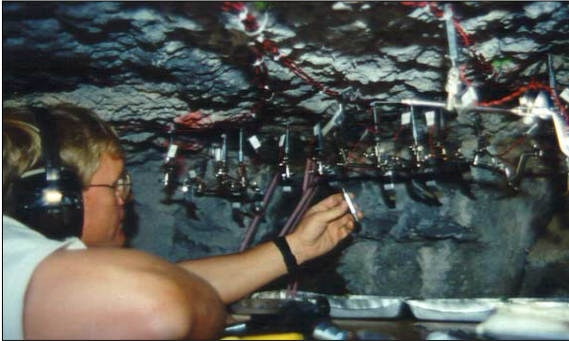
Figure A-3. Apparatus for measuring flow and transport in vesicular basalt at the Hell's Half Acre site.
