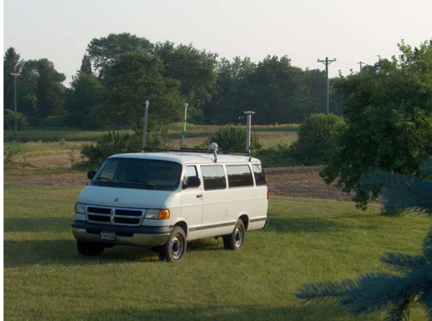
Figure 8. Van setup used for collecting data broadcast from HAG1 and HRN2, at the same time. Note one GPS marine antenna and two demodulator receiver antennas.
