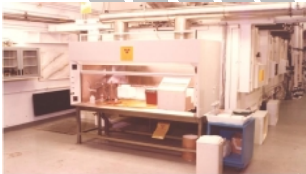
Shown here is part of the hot cell suite in the Medical Department where radioisotopes produced in the BLIP are processed for distribution to medical, industrial, and research users.
