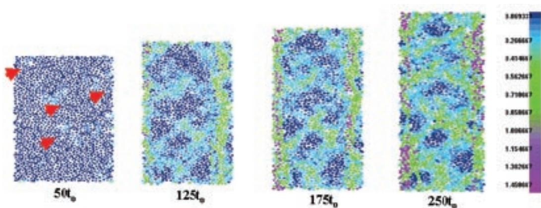
**This graphic representation shows the evolution of microstructure with time during deformation under constant stress. Atoms were colored depending on the strain they accumulated, and arrows indicate the location of the free volumes as observed during the MD simulations.**
