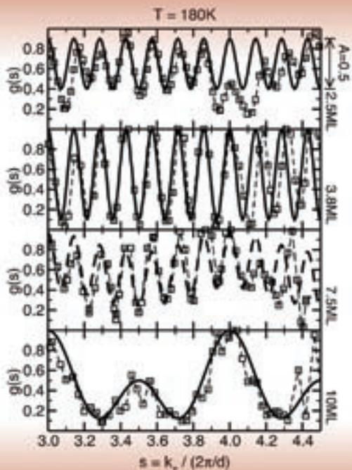
Electron diffraction “fringes” (similar to the ones formed when light scatters from a very thin air wedge, but of much larger size) can be used to deduce that practically all islands are seven layers high for lead coverages between 2.5 ML, or monolayers, and 7.5 ML.
