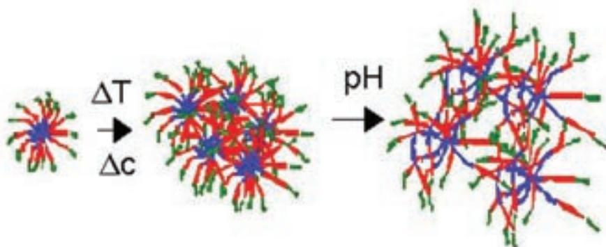
**This schematic shows how clusters, or micelles, of polymer strings group together as the temperature rises (center) and then respond to changes in pH (right). Each string is comprised of five blocks – one hydrophobic block (blue), two hydrophilic blocks (red) and two cationic blocks (green).**
