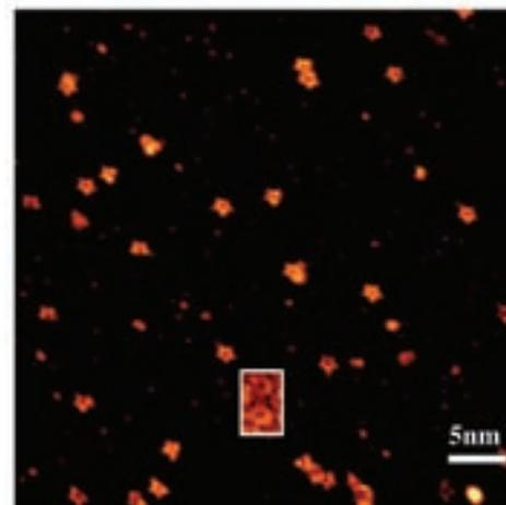
**This scanning tunneling electron micrograph of the quasicrystalline substrate shows how the atoms of aluminum, deposited using thin-film technology, gather in star-shaped clusters around 2 angstrom-deep holes. This site-specific nucleation and the fact that the “starfish” are uniform in size represents a breakthrough in the understanding of the surface characteristics of quasicrystalline materials.**
