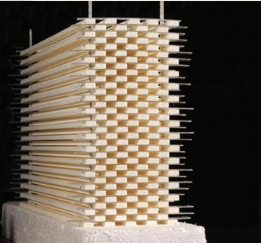
**This photonic crystal has a negative index of refraction equal to -1, providing excellent subwavelength resolution. A negative index of refraction equal to -1 is needed to achieve a perfect image.**
