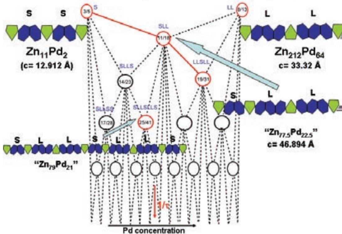
This diagram shows how Miller and Gourdon were able to use a Farey tree model to predict the unit length of different compositions of compounds in a zinc-palladium system. The top two compositions represent the “borders” of the quasicrystalline gamma brass phase and represent short and long one-dimensional atomic clusters. As the tree cascades down, the subsequent compositions are made up of corresponding combinations of short and long clusters.
