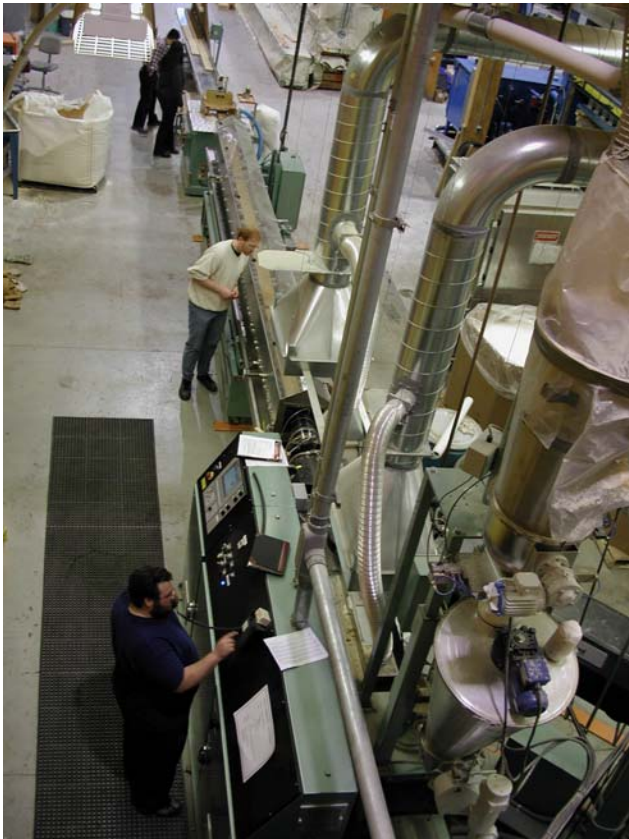
Figure 13: 94 mm profile extrusion line running formulation 1
