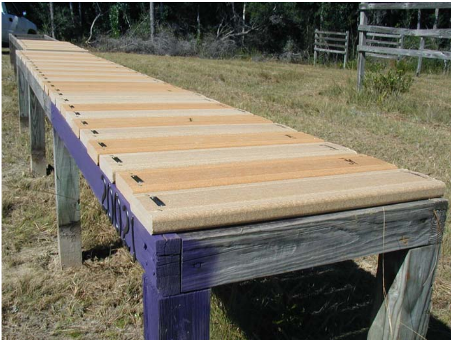
Figure 17: Deck boards installed in the Harrison Experimental Forest, Mississippi.
