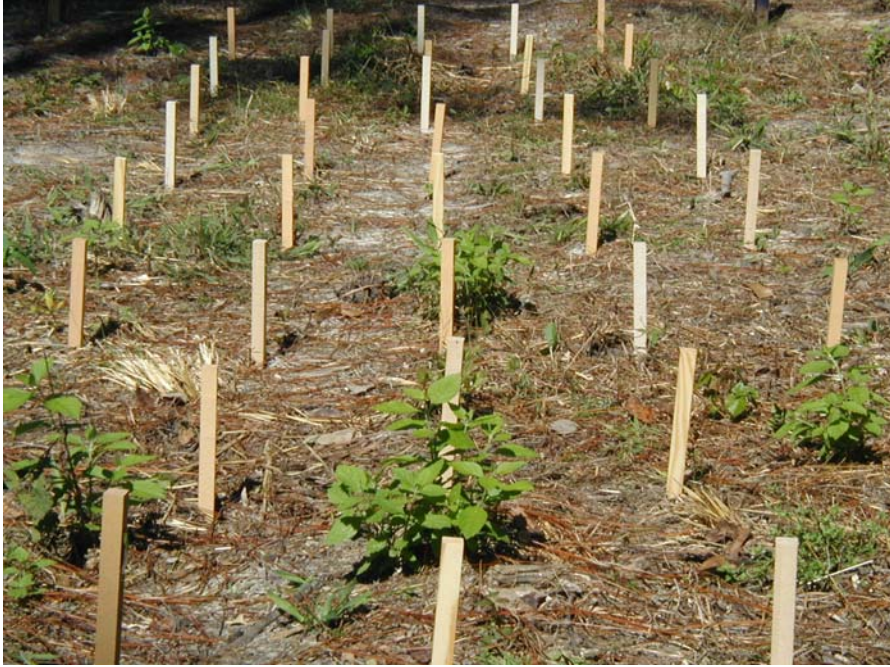
Figure 18: Ground stakes cut from deck boards installed in the Harrison, Experimental Forest, Mississippi.
