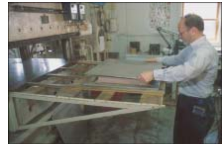
Jim Muehl, FPL Forest Products Technologist, demonstrates the process of creating a composite panel by blending the wood fiber and plastic together, forming a mat from the blended materials, pre-pressing the mat prior to hot-pressing, and loading the formed mat into the hot press to create the finished panel.
