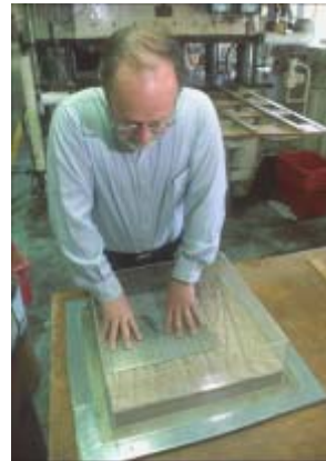
Jim Muehl, FPL Forest Products Technologist, demonstrates the process of creating a composite panel by blending the wood fiber and plastic together, forming a mat from the blended materials, pre-pressing the mat prior to hot-pressing, and loading the formed mat into the hot press to create the finished panel.
