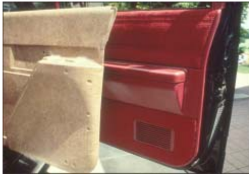
Wood–plastic composites are strong yet lightweight, making them ideal for the automotive industry.
