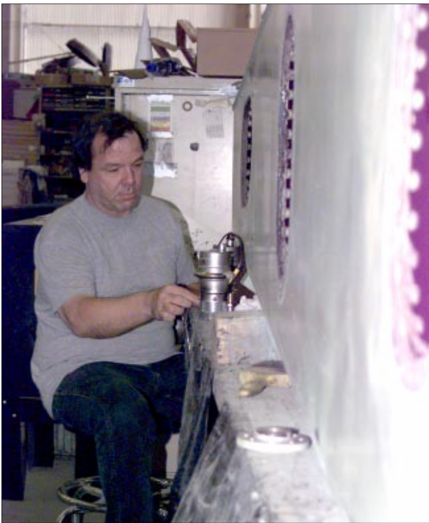
Bill Hamilton, heavy mobile equipment repair, replaces the seals and gaskets on a fuel cell.
