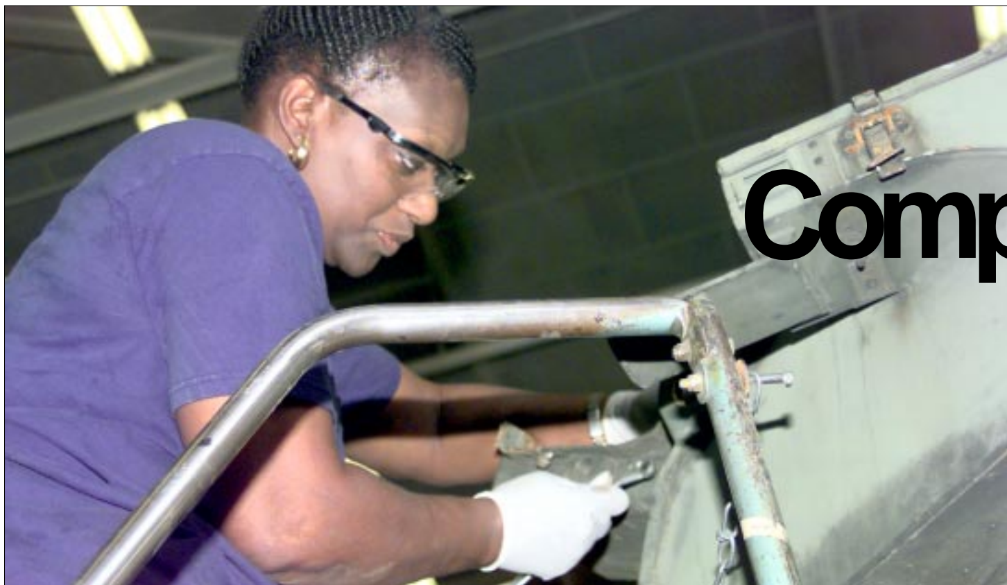
Lola Harris, artillery repair, dismantles parts from an AAV/P7 turret to inspect them for damage and wear.
