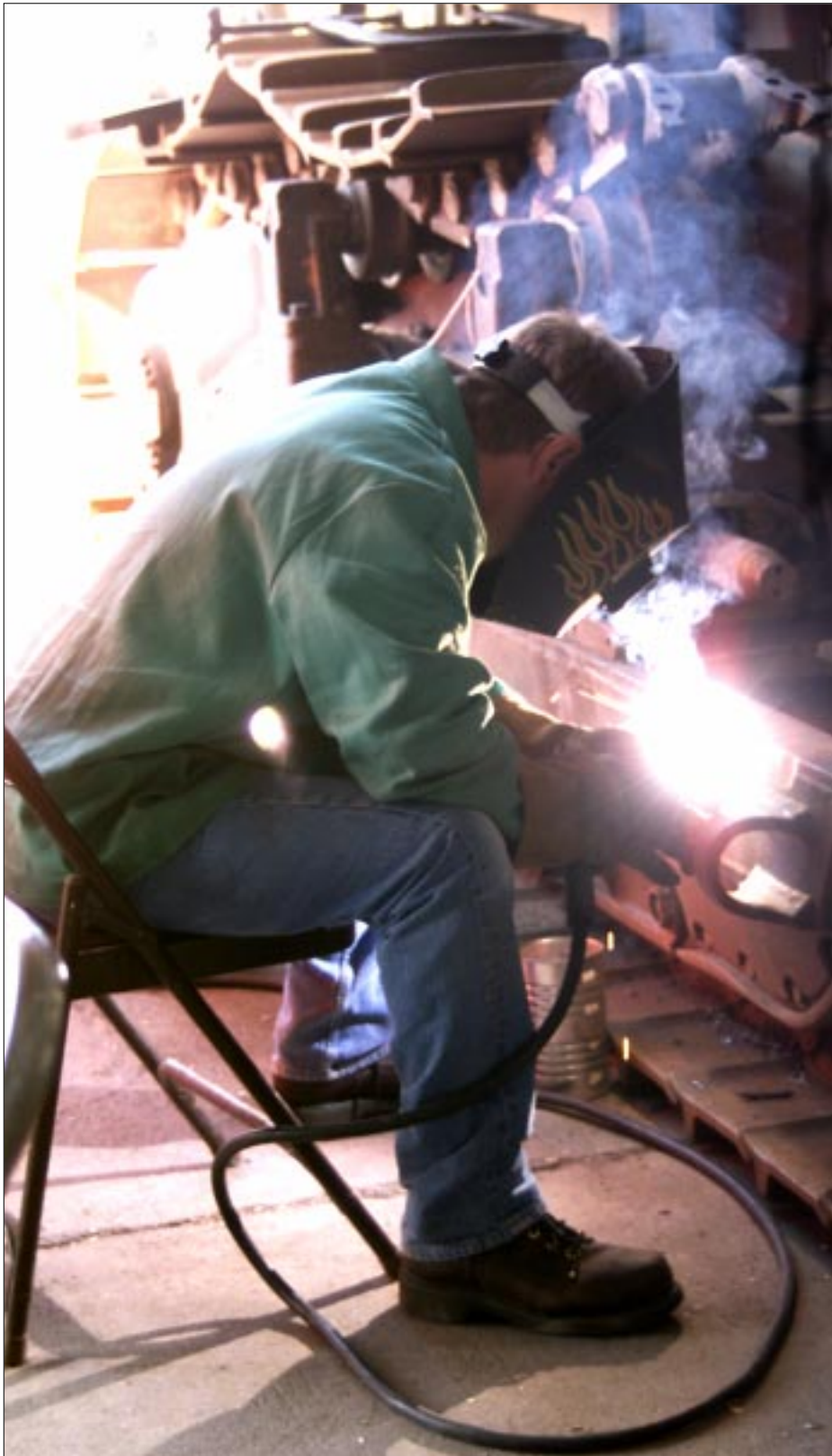
Greg Walsten mends the rail guides on a bulldozer; a three-day task from start to finish.
