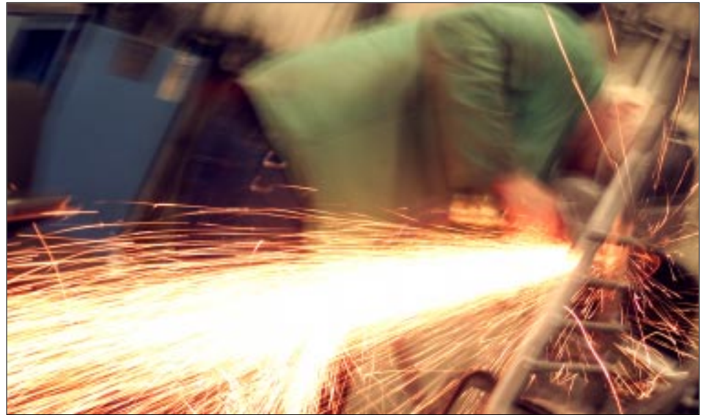
Welder Tom Pitard grinds a turret support for a Light Armored Vehicle.
