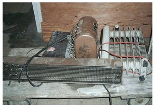
To the left are improper space heaters that were found in use in Congressional facilities. The space heaters are old and damaged and several were covered with rust. None of these space heaters were approved by a recognized laboratory for commercial use.
