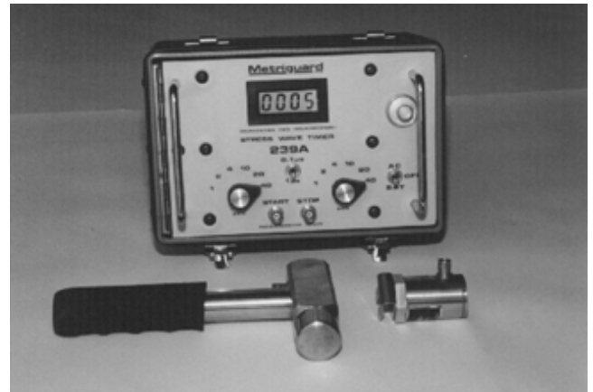
Figure 9—Metriguard Model 239A Stress Wave Timer.
