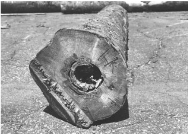
Figure 1—Decay and loss of wood material on butt end of log 1. (M93 30157-4)
