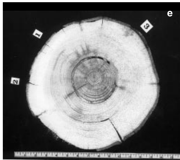
Figure 7—Log 1 tests. (a) Sound wave transmission times and corresponding velocity values; (b,c) CT scans at 6-in. (152-mm) and 36-in. (914-mm) positions; (d,e) photographs of sliced log corresponding to CT scans. 1 in. = 25.4 mm; 1 ft = 0.3048 m.
