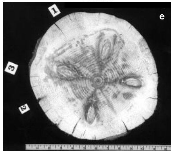
Figure 8—Log 2 tests. (a) Sound wave transmission times and corresponding velocity values; (b,c) CT scans at 30-in. (762-mm) and 72-in. (1,829-mm) positions; (d,e) photographs of sliced log corresponding to CT scans.
