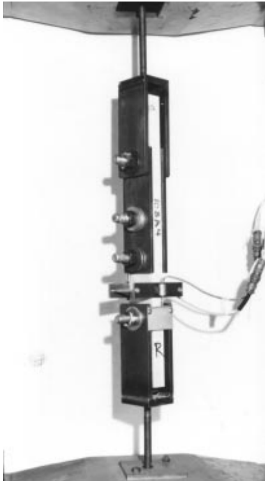
Figure 2—Test setup for tension parallel-to-grain connection tests.
