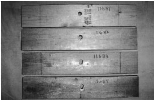
Figure 1—Specimens having (top to bottom) no reinforcement and one, two, and three layers of fiberglass reinforcement.
