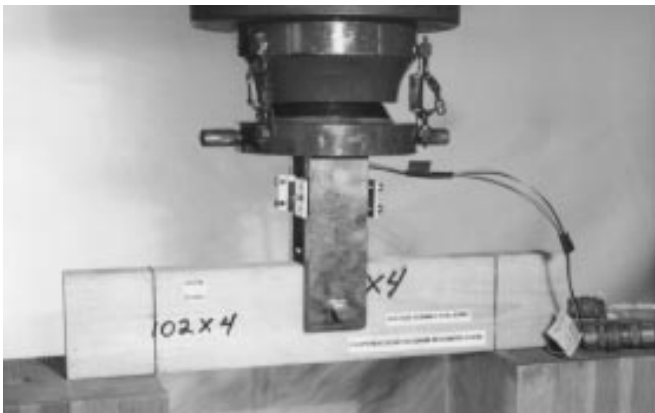
Figure 3—Test setup for compression perpendicular-to-grain connection tests.
