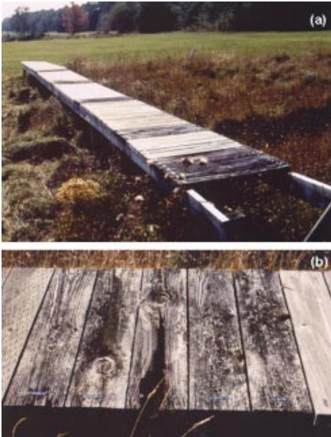
Figure 1—Aboveground field trials: (a) view of entire test deck; (b) close-up of portion of deck.
