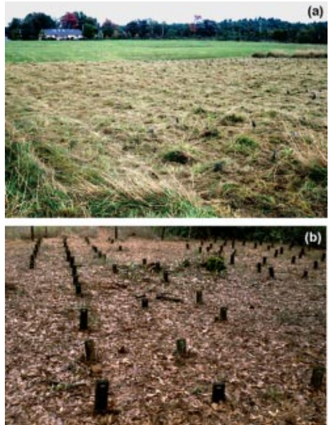
Figure 2—Ground-contact field trials: (a) exposure site; (b) test stakes.
