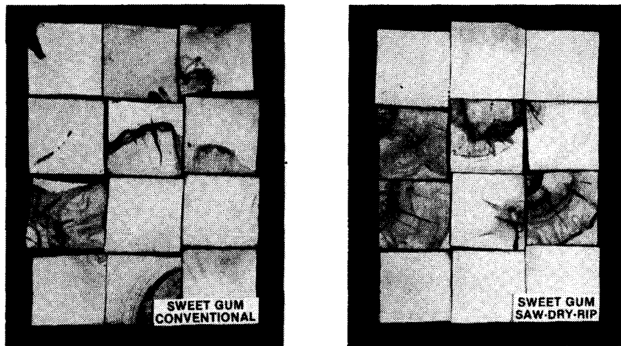
Figure 7.--Samples of sweetgum turning squares manufactured by conventional and SDR processes and dried in a vacuum-dehumidification kiln. (M 86 0117-18)
