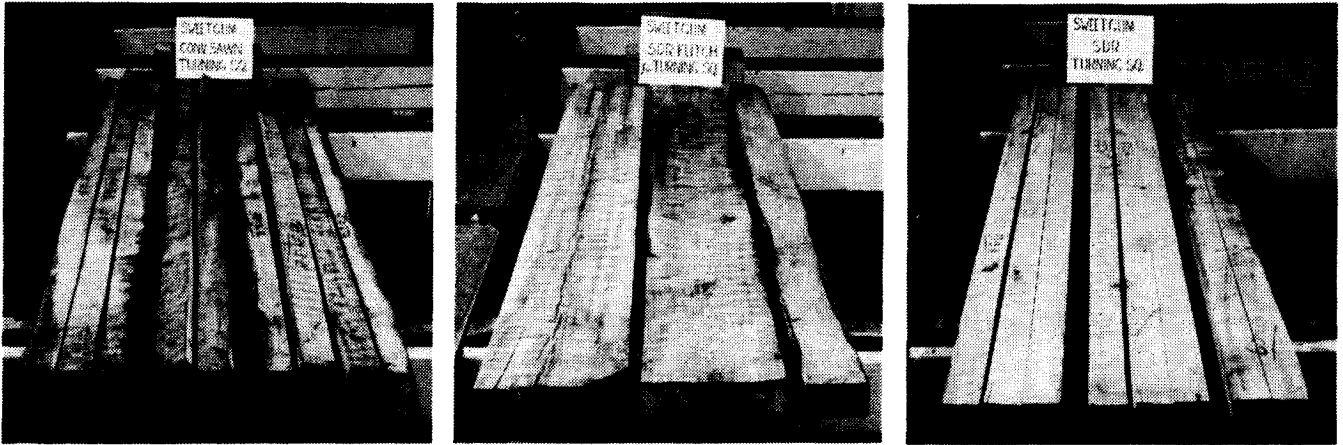
Figure 4.--Examples of sweetgum turning squares. a. Conventionally sawn squares cut green and dried. (M86 0097-5) b. SDR flitches before ripping. (M86 0099-5) c. SDR squares after ripping. (M86 0099-6)
