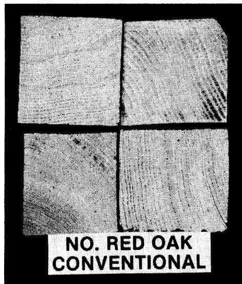
Figure 5--Samples of northern red oak turning squares dried in the vacuum-dehumidification kiln. (M 86 0116)
