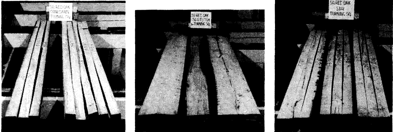
Figure 2. --Examples of southern red oak turning squares. a. Conventionally sawn squares cut green and dried. (M86 0088-3) b. SDR flitches before ripping. (M86 0088-6) c. SDR squares after ripping. (M86 0089-2)
