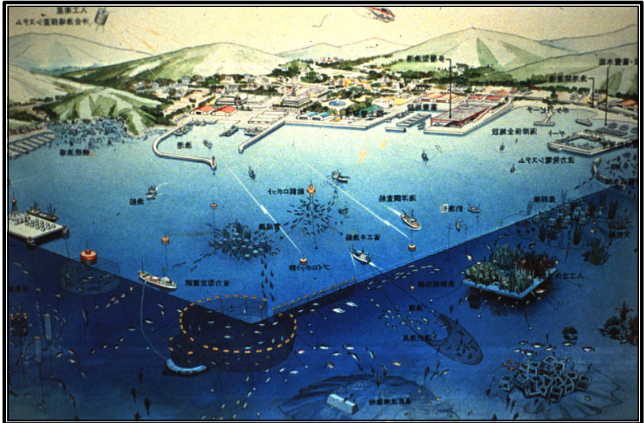
(Fig. 17) Those are typical artificial fish reefs for fish aggregation and propagation purposes.
