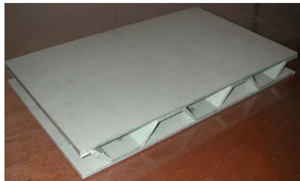
Finished thickness of corrugated panels could be around 1\frac{1}{2} inches.
