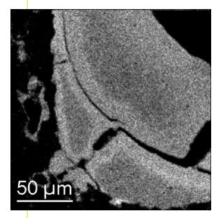
Platinum X-ray map from a sample loaded with platinum after 500 desulfation hours. Note the higher concentration of platinum at free surfaces in the washcoat, which remained essentially constant with aging treatments. High Temperature Materials Laboratory • Catalyst Characterization
