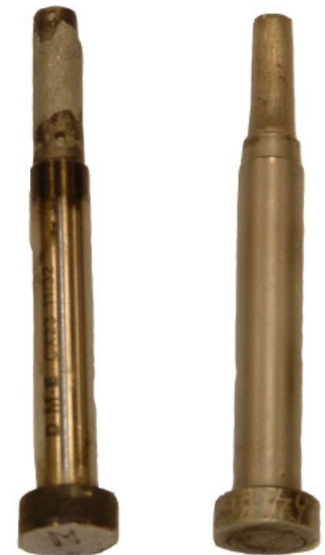
H-13 steel die pins removed from same mold. The untreated (left) and treated (right) pins after 3,500 and 200,000 shots of aluminum, respectively.
