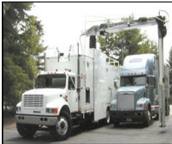
Digital imaging of truck trailer contents
