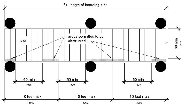
Figure 1003.3.2 Boarding Pier Clearance
