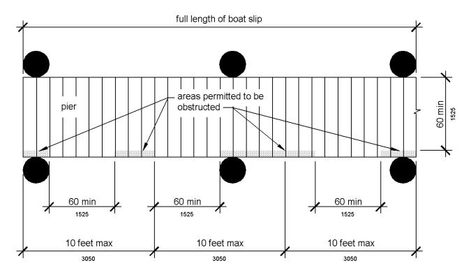
Figure 1003.3.1 Boat Slip Clearance
