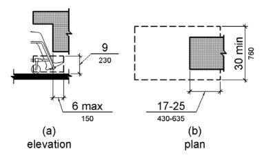
Figure 306.2 Toe Clearance
