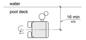
Figure 1009.2.2 Pool Lift Seat Location
