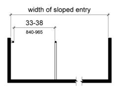
Figure 1009.3.3 Handrails for Sloped Entry
