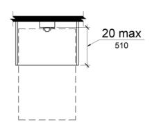
Figure 704.2.1.2 Forward Approach to Telephone
