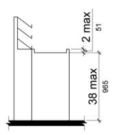
Figure 904.3.2 Check-Out Aisle Counters
