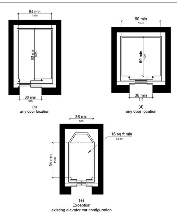
Figure 407.4.1 Elevator Car Dimensions
