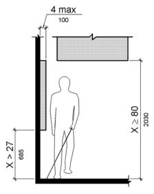
Figure 307.2 Limits of Protruding Objects
