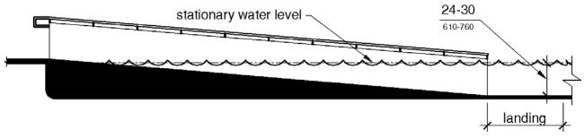
Figure 1009.3.2 Sloped Entry Submerged Depth
