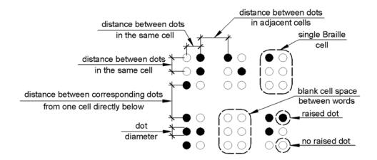
Figure 703.3.1 Braille Measurement
