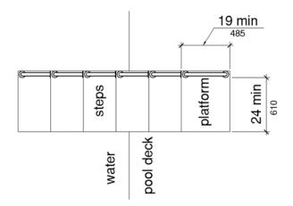
Figure 1009.5.1 Size of Transfer Platform
