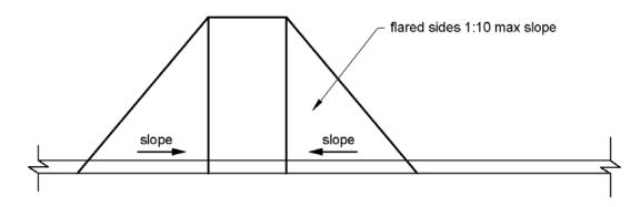
Figure 406.3 Sides of Curb Ramps
