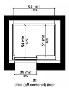
Figure 407.4.1 Elevator Car Dimensions
