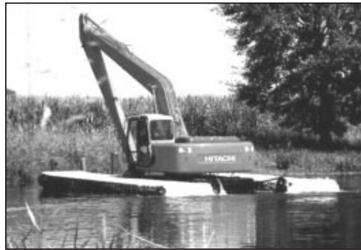
The Pacific Islands Team is planning to use an aquatic excavator to remove aquatic invasive species.
