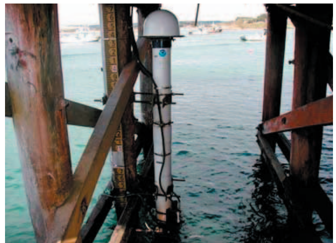
Figure 5. Stilling well holding the Druck sensor and 436B encoder assembly.
