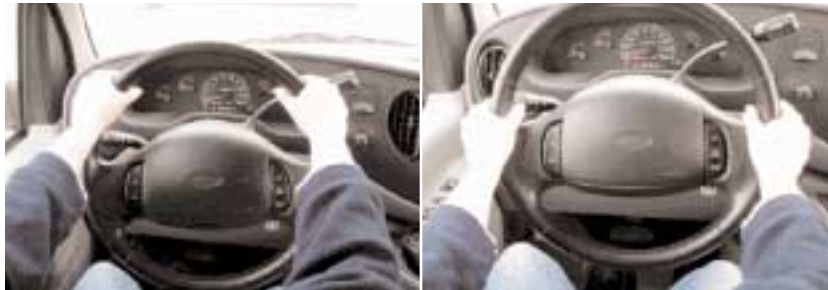
Air bags have altered safe steering wheel hand positions. The incorrect positions, left, result in injury when bags deploy. The correct positions, on right, keep hands and lower arms clear of the deploying air bag.
