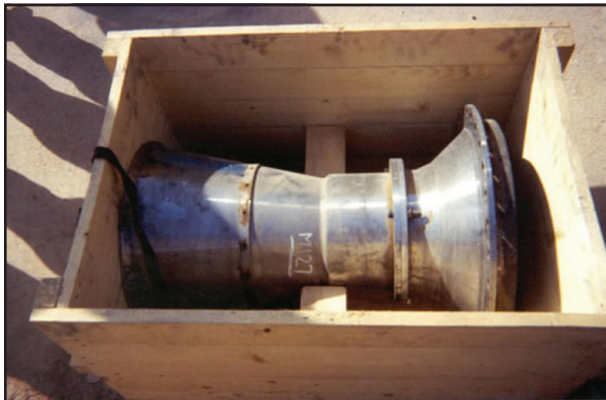
Figure 15. Al Fat'h rocket motor nozzle.
