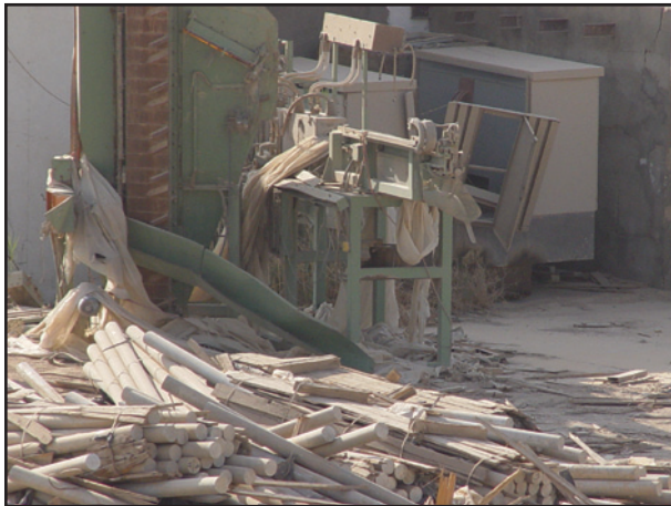
Figure 13. Dispersed and destroyed flow-forming machines (Tho Al Fiqar).
