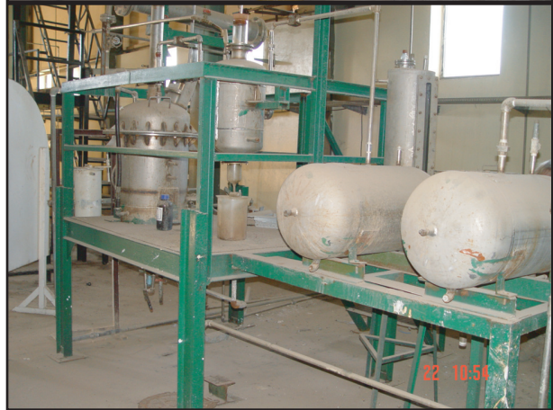
Figure 41. Spray dryer and other process equipment in Building 53.
