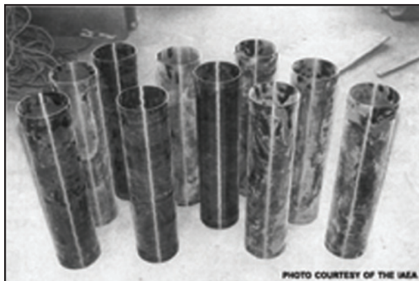
Figure 10. Carbon fiber tubes.
