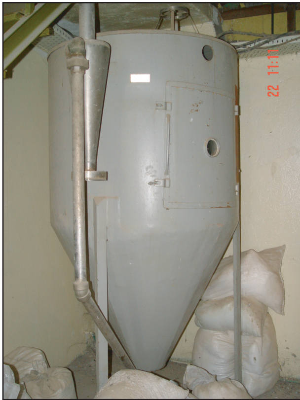
Figure 41. Spray dryer and other process equipment in Building 53.
