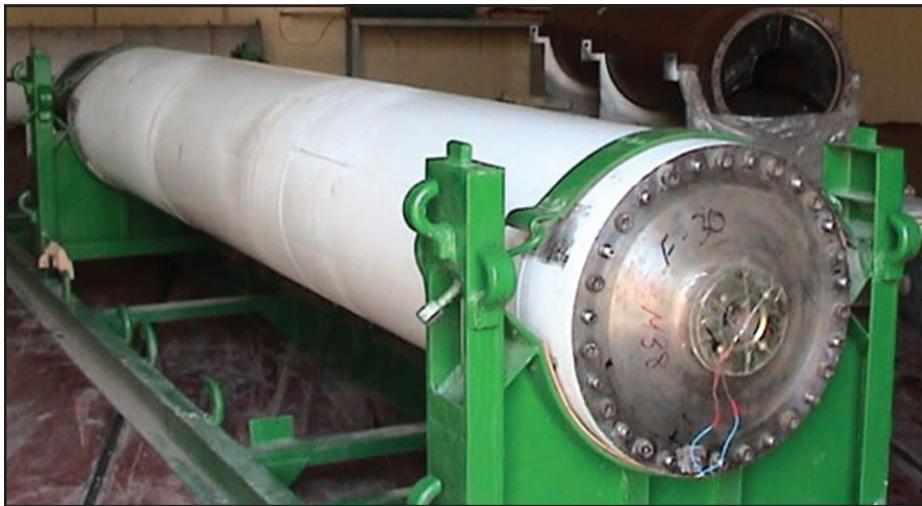
Figure 7. Al Fat'h solid rocket motor.
