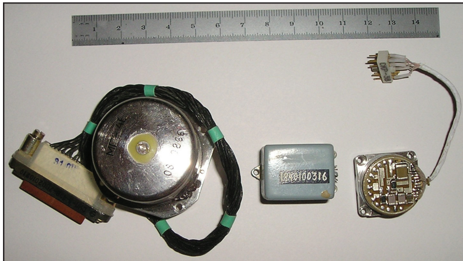
Figure 28. MG-4 gyroscope, AK-5 and A-15 accelerometers.
