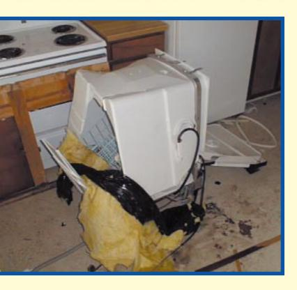
gas. They suspected the bulk of the gas was a combination of hydrogen and oxygen, which was generated by electrolysis in the hot-water heating systems.
