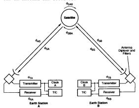
3. Two-way time transfer using a satellite.
