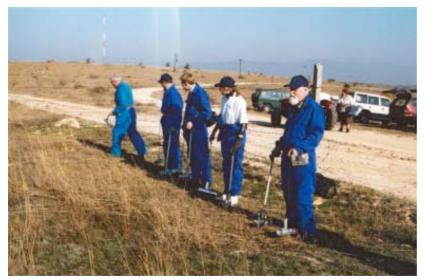
radiation in the environment were made using beta and gamma instruments held close to the ground, with the team members often employing the 'line-up' survey technique described in С Appendix 'Methodology and Quality Control'.
