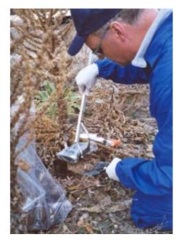
Beta and gamma measurements on soil sample from penetrator hole at Pljackovica
