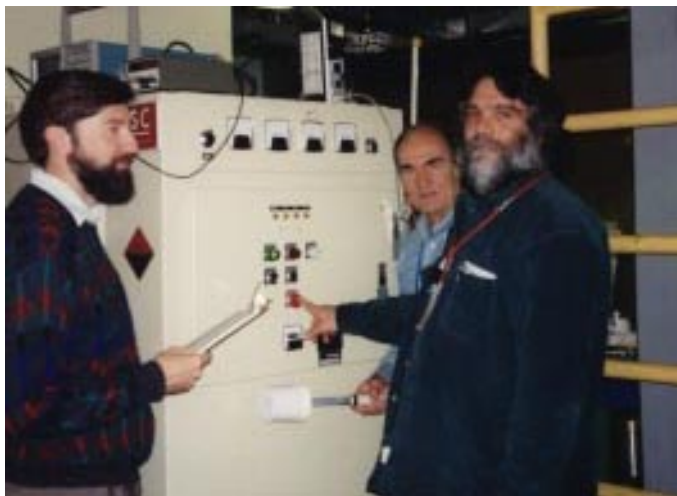
A radio frequency oven from the U.S. Department of Agriculture (USDA) is presently at PPPL for testing and modifications as part of a collaborative project between PPPL and the USDA to develop new pasteurization methods that use radio frequency (RF) waves and microwave heating. Next to the oven are members of the PPPL team, including (from left), Chris Brunkhorst, Elmer Fredd, and Dave Ciotti. Not pictured is Randy Wilson. The machine is expected to be returned to the USDA's Eastern Regional Research Center in Philadelphia sometime this summer, where the pasteurization experiments will take place.
