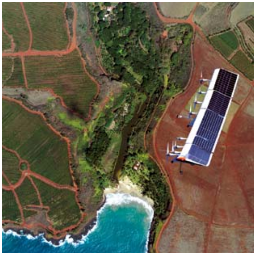
Ames Earth Sciences research activity using a Solar-powered Pathfinder Plus Unmanned Aerial Vehicle (UAV) with a Clark University multispectral camera imaging Hawaiian coffee fields in an effort to optimize the harvest of the richest coffee beans.
