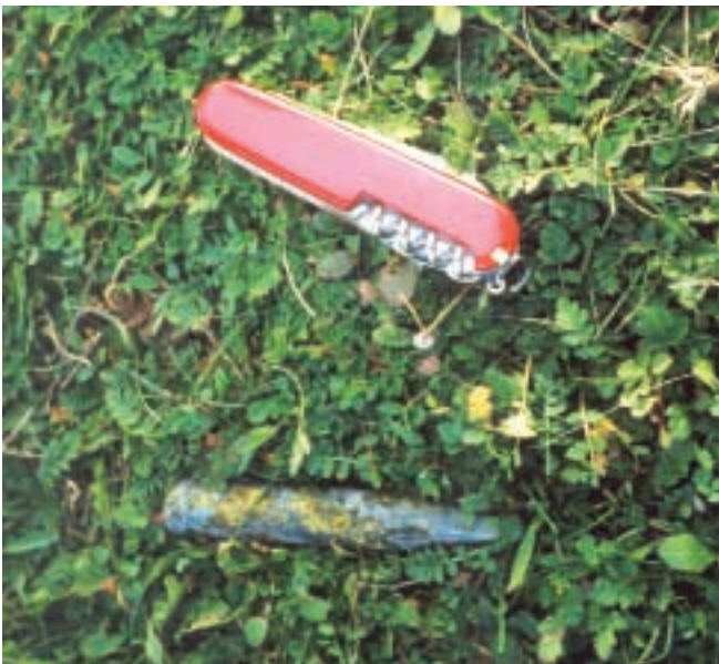
A penetrator found lying in the grass. Note the yellow coating on the penetrator. Planeje/Planeja.
