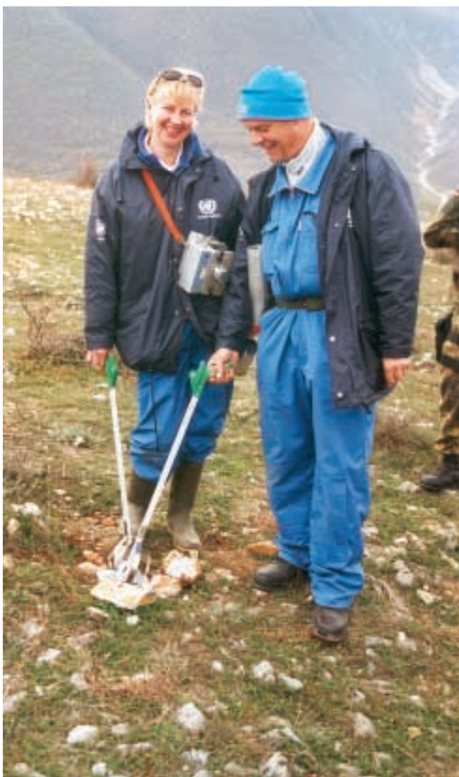
Measurement of beta radiation with the Inspector instrument wrapped in a plastic bag and held close to the ground. Ceja mountain.
