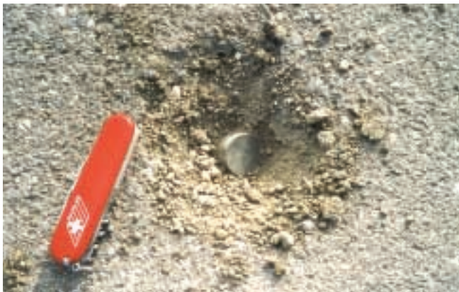
The jacket remained in the hole and the penetrator continued into the soil beneath the asphalt layer.
